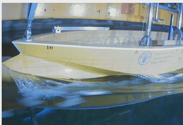
Testing of a longliner with an FAO-designed dihedral bow retrofit, Sri Lanka © FAO/Francisco Pérez Arribas
